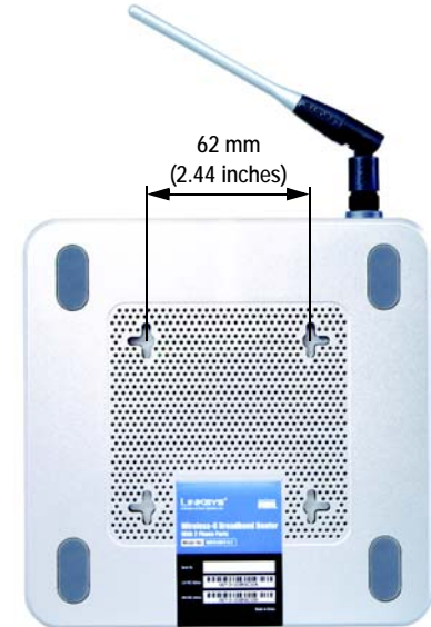
Figure 4-6: Measurement between Wall-Mount Slots
