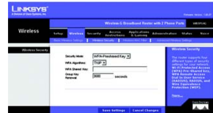
Figure 5-12: Wireless Tab - Wireless Security (WPA-Preshared Key)
